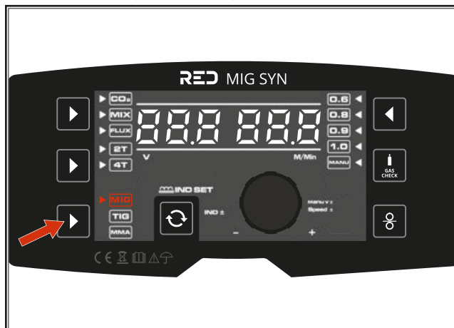
Fig. 9: Setting the welding process
