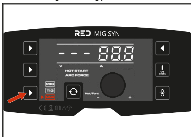
Fig. 21: Setting the welding process
