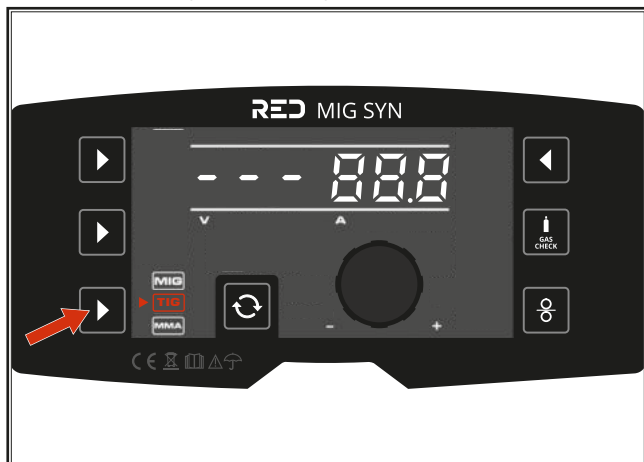
Fig. 19: Setting the welding process
